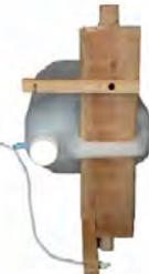
**4** Place yoke between supports and connect the yoke to the forearm lever with a nylon cord
